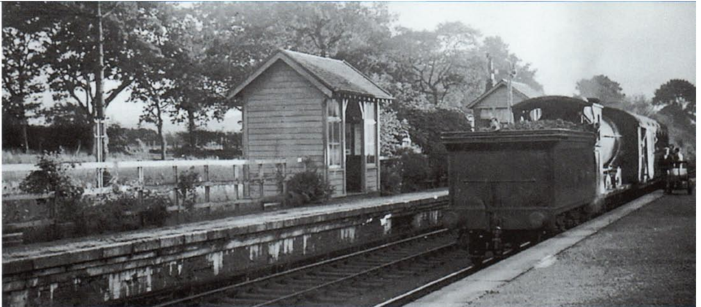
NBR Class J37 0-6-0 No.64598, running tender first, calls at Balfron on 18th September 1951 while working the Blanehead–Aberfoyle passenger shuttle service. Parcels are being unloaded from the single Gresley brake composite non-corridor suburban coach. (G. H. Robin)
